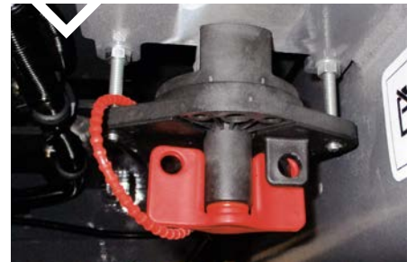
KEY-LOCKABLE SWITCH FOR DISCONNECTION OF THE ELECTRICAL ENERGY
