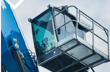
CATWALK WITH HANDRAIL*
