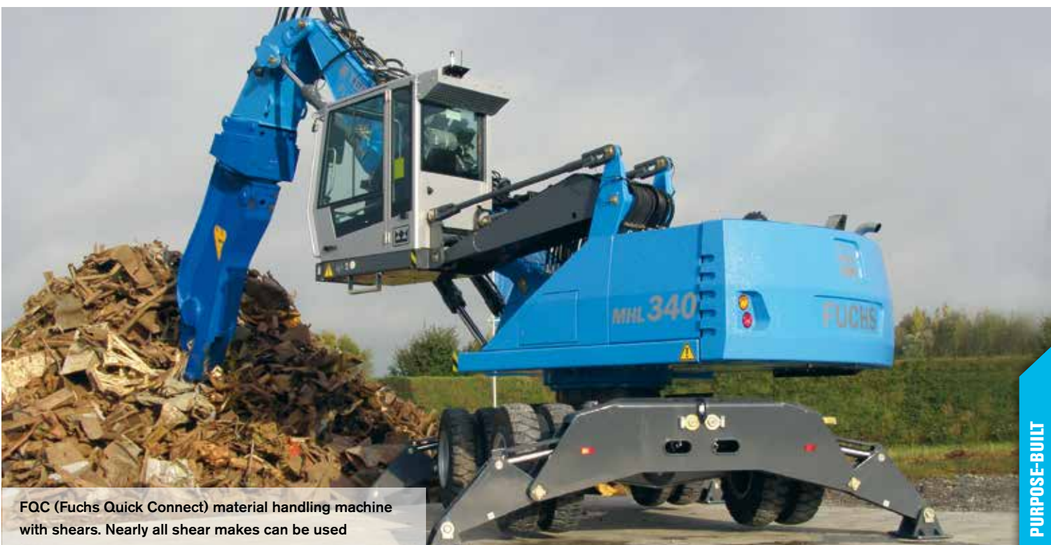
Larger stabilizer pads for a lower ground pressure
