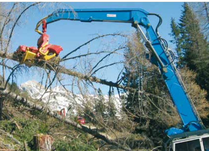
MHL380 superstructure with offset cab mounting
