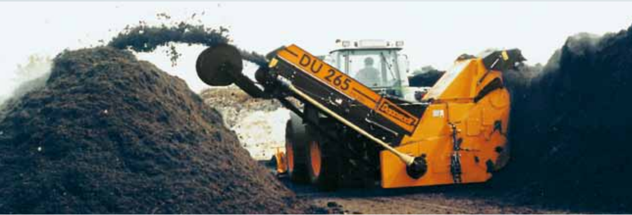
Turning and ventilating of a windrow
