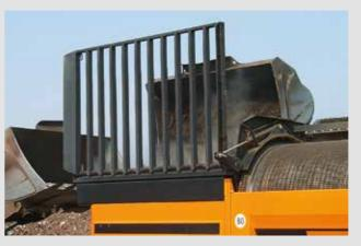
The stonegrid enables the separation of bulky contaminants (e.g. big rocks) and prevents damage, e.g. of the drum. The stonegrid is tilted hydraulically via remote control. The material is tipped at the left side of the machine.
