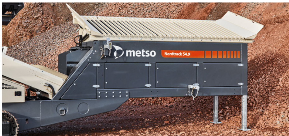
Robust tipping grid with remote controllable tilting. Possibility to offer also vibrating grid
